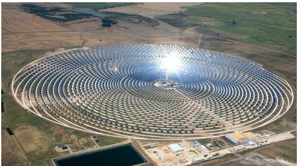
A Concentrated Solar Plant That Uses Mirror-Lenses
